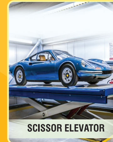
SCISSOR LIFT WITH LOAD BEARING ROOF
